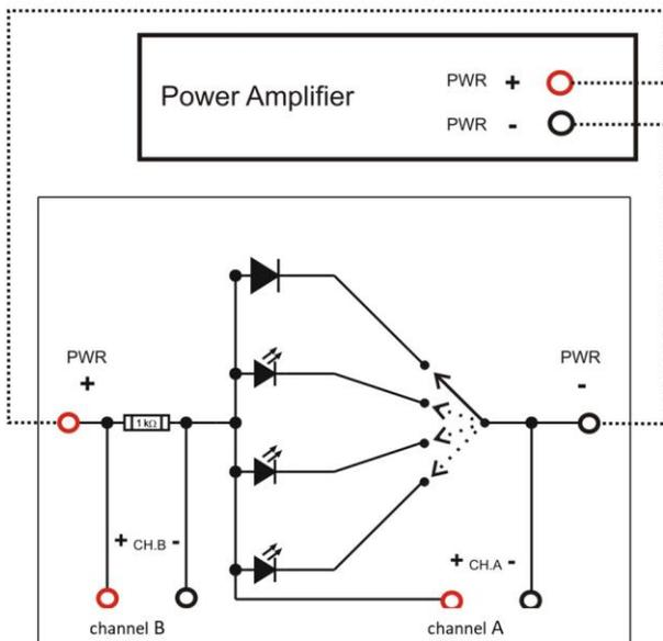
Fig. 5 Diode circuit wiring diagram. Part P46.
