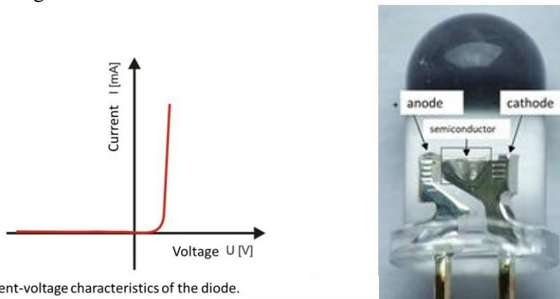
Fig. 4 Current-voltage characteristics of the diode.
